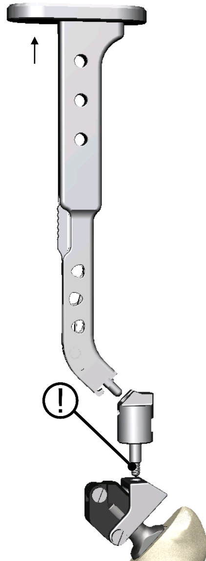
Figure 10: Stem-repositioner with Rasp handle straight and Adapter modular in necessary alignment to the implant
